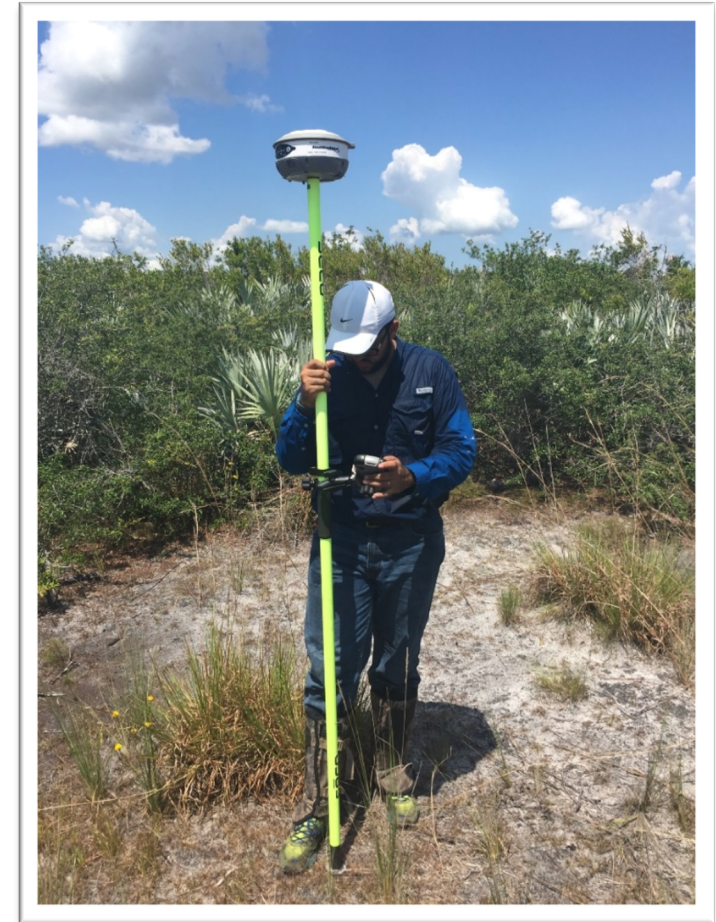
Felix Santiago-Collazo (PhD Student, LSU) using RTK-GPS survey equipment.
